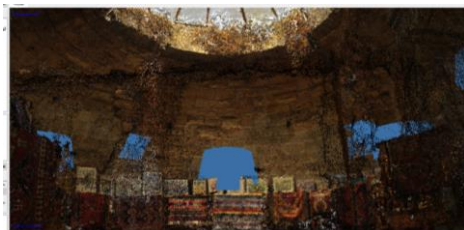
Fig. 12- Dense point cloud of the tower (Griffo, 2017).
