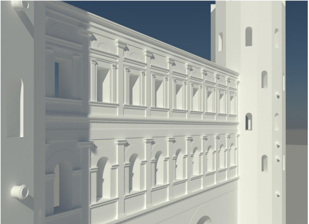
Fig. 6 – Render of the three-dimensional model of the Porta Palatina : overview and detail of the two-horizontal partition of the interturrio .
