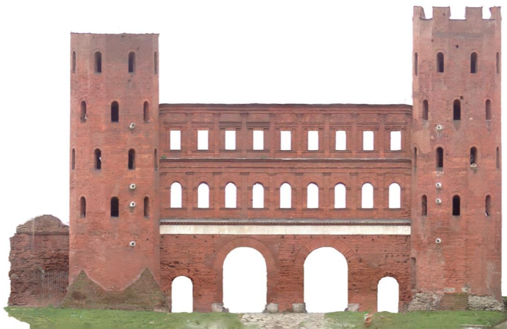
Fig. 3 –Orthomosaic of the north elevation of the Porta Palatina, produced starting from the texturized model using photoscan® (author).
